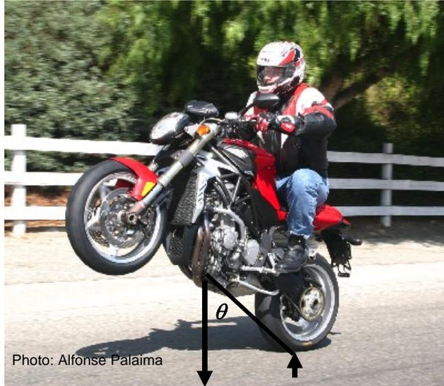
To loft the front wheel into the air, the rider must do something to upset this equilibrium, i.e. they must unbalance the torques about the rear wheel.
